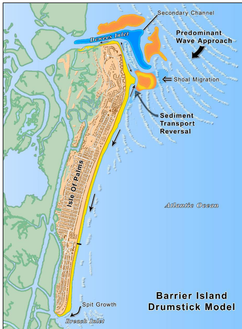
FIGURE 1. "Drumstick" barrier island model developed from Hayes (1979).
