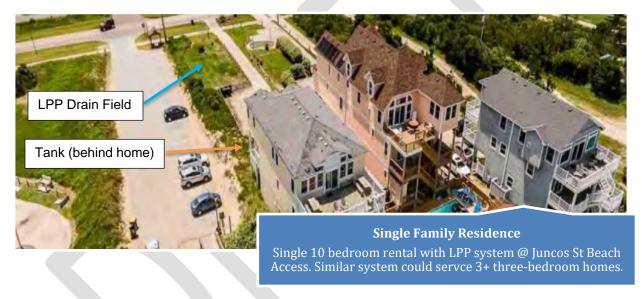
Figure C- 1. Examples of large and/or advanced onsite wastewater systems at large residential sites that provide analogous treatment scale or volume to smaller-scale or clustered residential decentralized cluster system opportunities.
