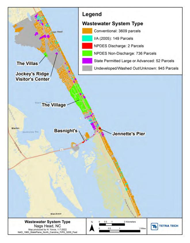
Figure 7-2. Wastewater System Types in Nags Head
