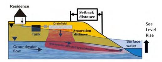
Figure 8-1. Influence of sea level rise and rising groundwater tables on septic systems in coastal settings
