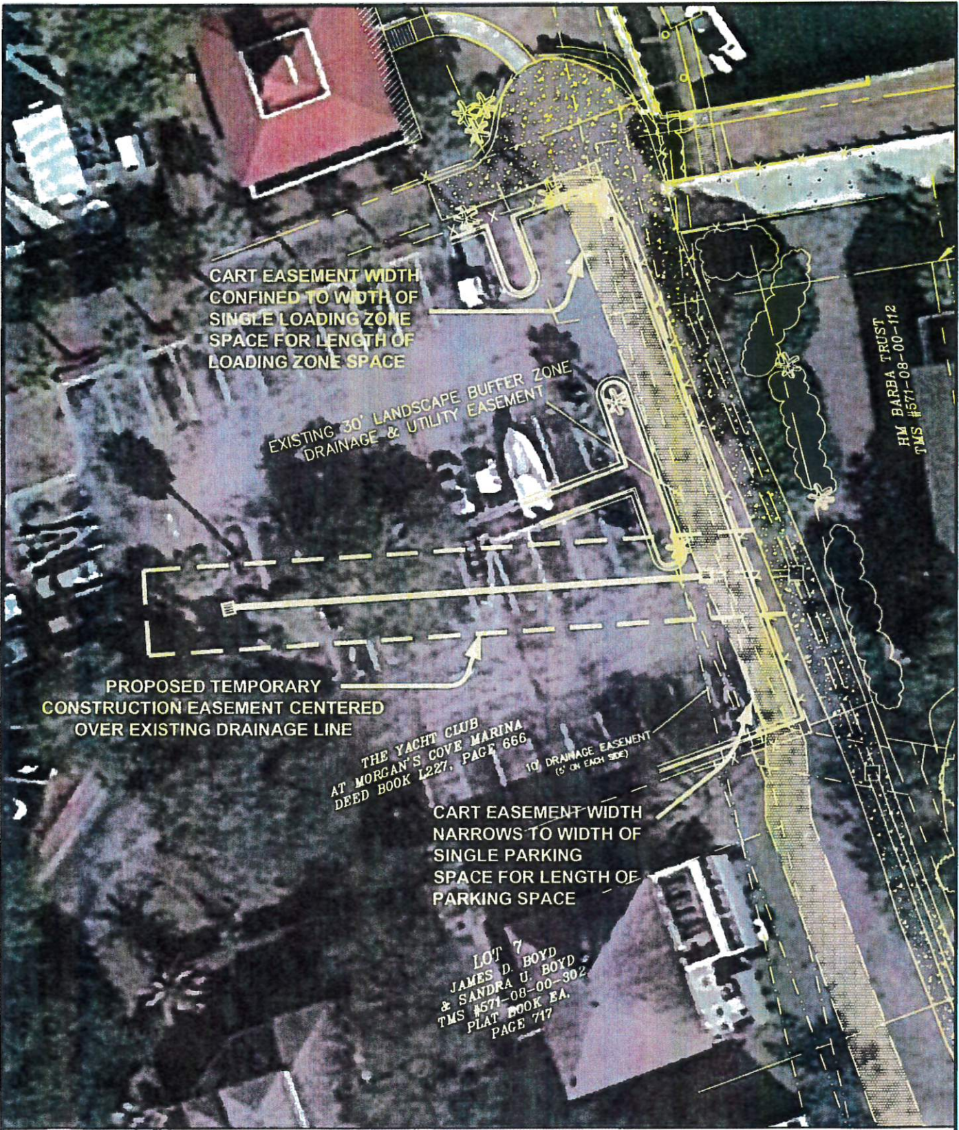
EXHIBIT SHOWING A TEMPORARY CONSTRUCTION EASEMENT ACROSS THE PROPERTY OF THE YACHT CLUB AT MORGAN'S COVE MARINA
