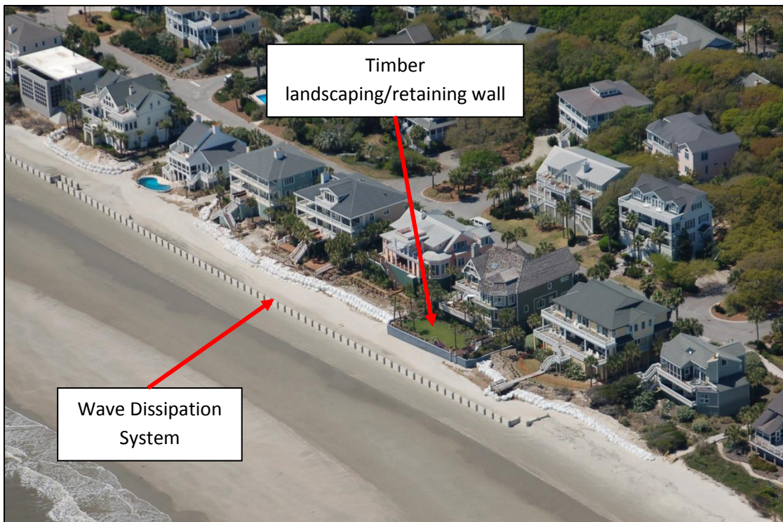
Figure 20. April 5, 2016 photo of Wave Dissipation System installation at Beachwood East (same area as shown in Figure 16). WDS ties into rock revetment at west end, see Figure 19. A timber retaining/landscaping wall is also shown. The Wave Dissipation System was removed in 2018.
