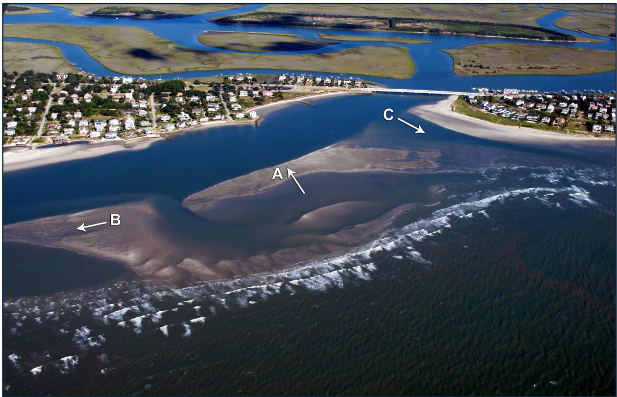
FIGURE 3.35. Aerial images of Breach Inlet in April 2011 (upper) and September 2012 (lower). Note the buildup of the exposed shoal at A, seaward expansion at B, development of a marginal flood channel at C. A recent channel avulsion event is reaching its final stage, where the old channel (labeled) is completely infilled with sand (S) which was originally on the IOP side of the inlet. [Photos by TW Kana and SB Traynum]
