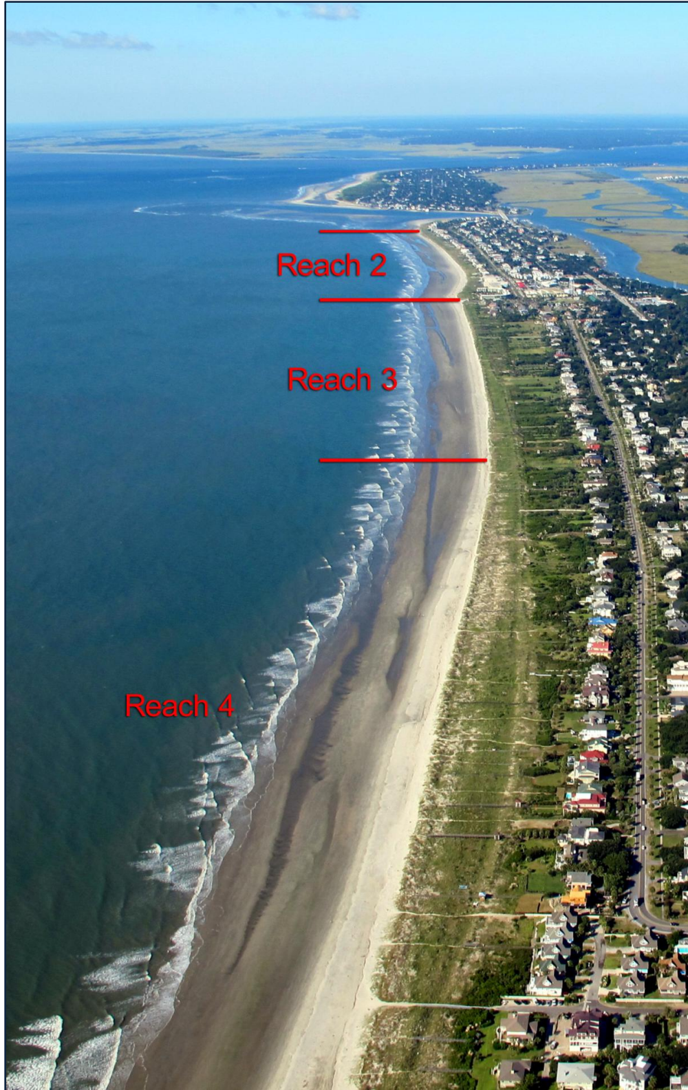
FIGURE 3.28. Aerial view of central and southern Isle of Palms on 25 September 2012. Properties in Reach 3 and Reach 4 are set back a few hundred feet from the beach. The seaward edge of the wax myrtles (dark green vegetation) marks an earlier foredune/shoreline position. [Photo by SB Traynum]
