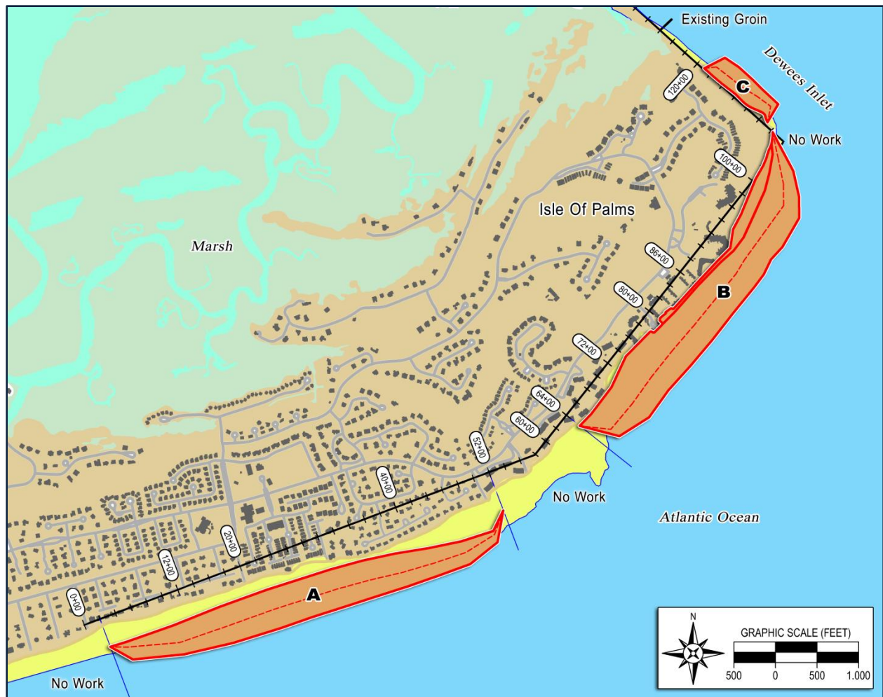
FIGURE 3.42. Reaches for the 2008 nourishment project. The graphic shows the project baseline with 0+00 located at 53 rd Avenue (monitoring station 222+00).
