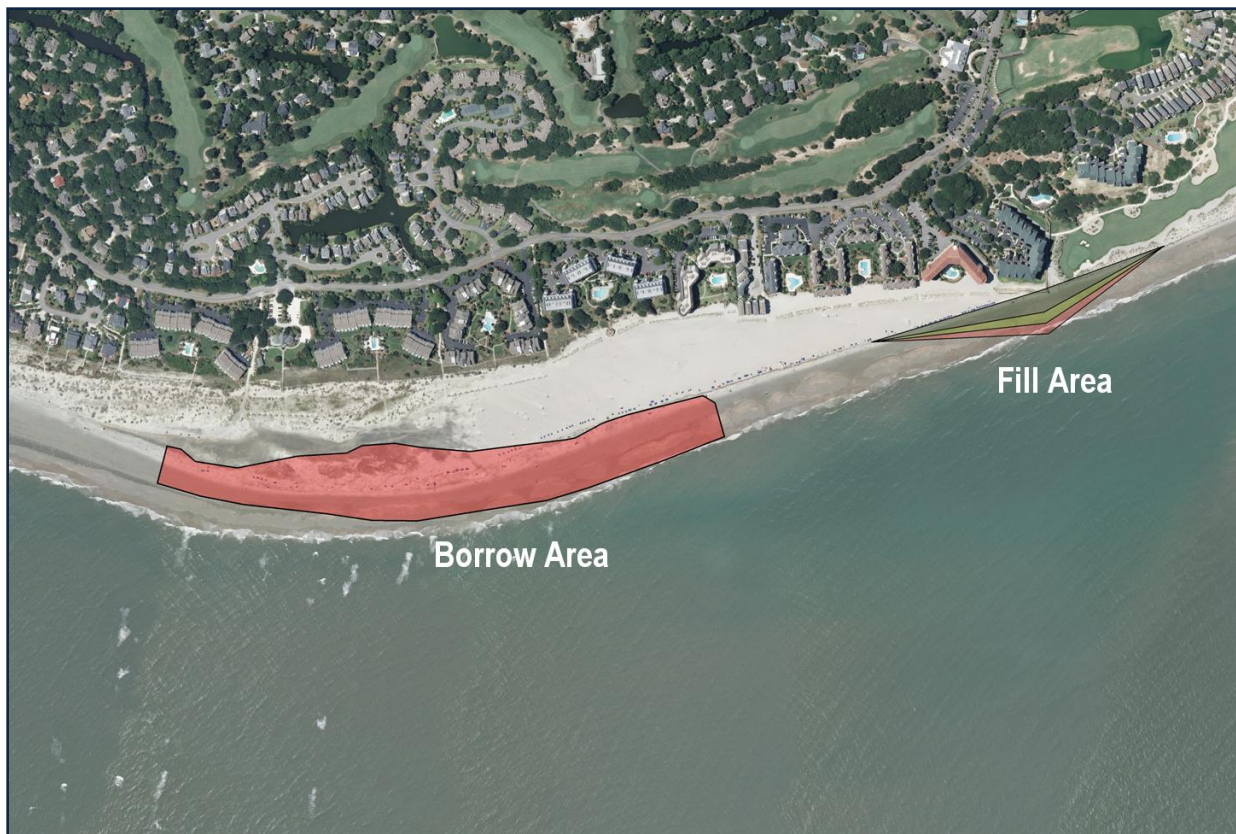
FIGURE 1. General project plan showing the borrow and fill areas. Aerial image (July 2011) courtesy IMC Inc (Charlotte NC).
