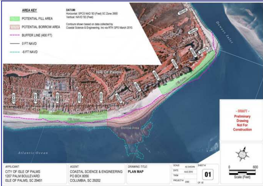
FIGURE 4. March 2010 aerial image of the northeastern end of Isle of Palms. General location of the potential excavation and fill areas under the current beach condition are shown. Only portions of the northeastern fill area are currently eroded beyond the 100-ft trigger line.
