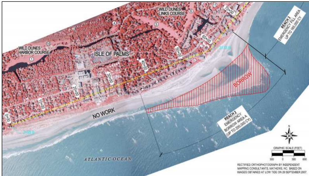
FIGURE 3. Example excavation area from a 2007 beach condition scenario. (Note that the cross-shore limits are different from the proposed buffer lines in this example, taken from CSE 2007.) A potential fill area is shown in Figure 5.
