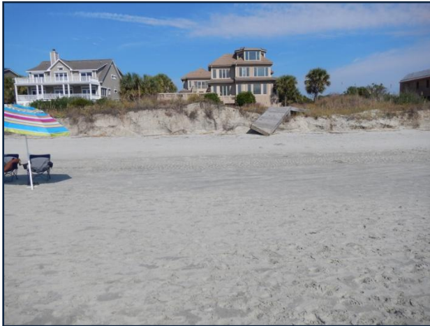
October 2013 (left) and January 2014 (right) images from station 8+00, looking toward the dune. The escarpment in this area moved a few feet landward between the image dates.
