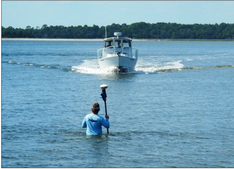
FIGURE 3.2. Surveying beach profiles involves collection of land-based data at low-tide and hydrographic data collection overlapping the land-based work.
