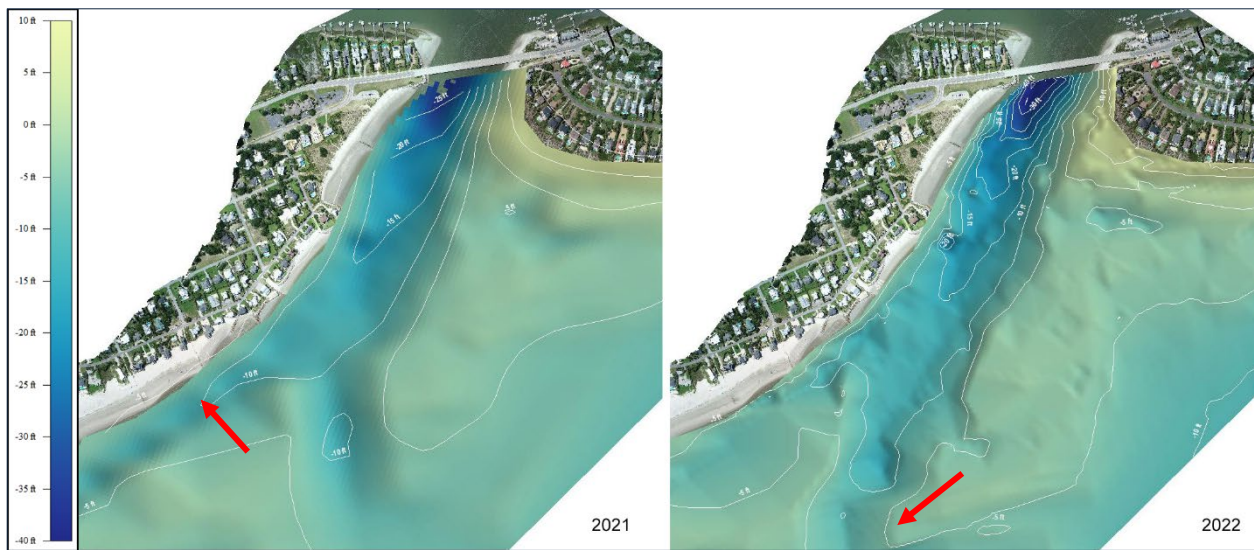
FIGURE 4.29. A pair of digital terrain models spanning the majority of the Breach Inlet channel collected in 2021 (left) and 2022 (right). The model shows the old main channel present in 2021 has infilled and the secondary channel has become the new main channel. No significant changes were observed along the northern shoal; however, it is elongating, which may draw sand off of Isle of Palms.
