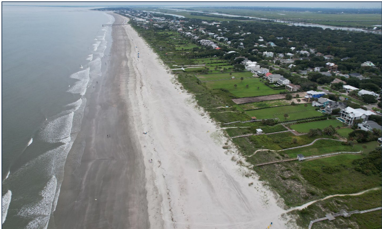
FIGURE 4.21. Aerial photo of Reach 3 in August 2022 (29 th Ave in the foreground). The long-term trend for Reach 3 is stable to accretional. Dwellings in the reach are generally set back from the beach between 400 ft and 500 ft.
