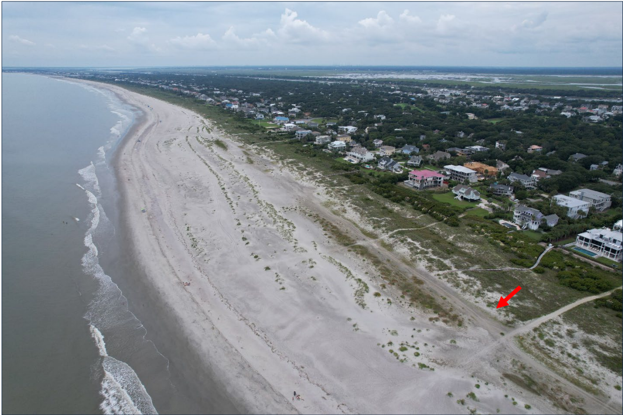
FIGURE 4.18. August 2022 aerial photo of Reach 4 (53 rd Avenue is at the right of the image). By being positioned downdrift of the nourishment area, Reach 4 receives nourishment sand spreading from the placement area as well as spreading shoal sand. This reach has gained sand every year since 2009 except 2016. As the vegetated dunes expand, sheltered locations (such as low-lying areas behind protective dune ridges) will gradually transform into a shrub habitat with larger areas of wax myrtle replacing dune grasses. The 2008 dune line is shown by the red arrow.
