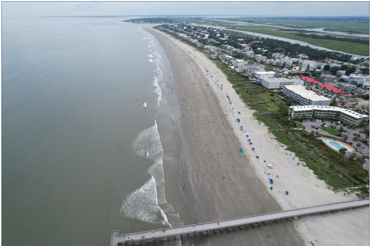
FIGURE 4.26. Aerial views of Reach 2 in Aug 2022. Since monitoring began in 2009, Reach 2 has been the most stable reach, typically showing lower magnitudes of volume change compared to the other reaches along Isle of Palms. The arc in the shoreline west of the pier indicates that the pier may act to trap sand, which may impact Reach 2 in certain wave conditions.
