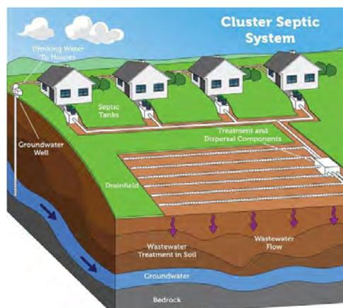
Figure 6-4. Decentralized Cluster System Layout, ref. US EPA
