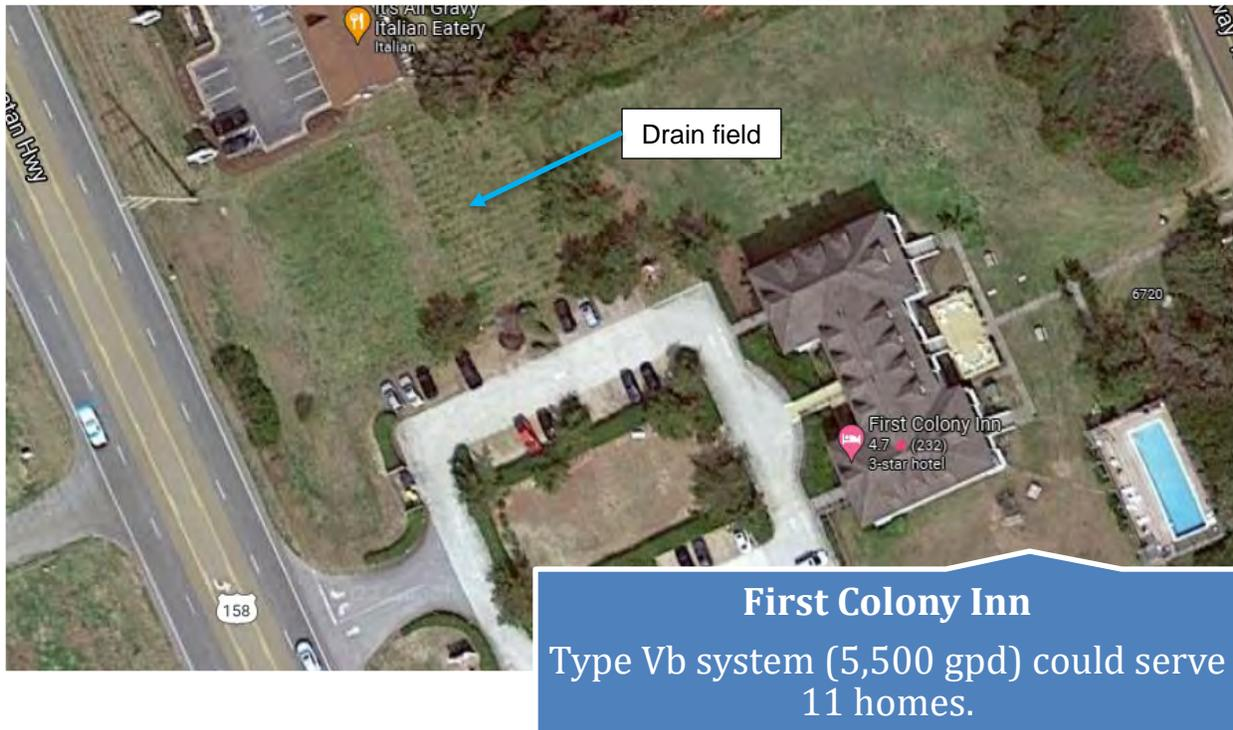
Figure C- 3. Examples of large and/or advanced onsite wastewater systems at hotel sites that provide analogous treatment scale or volume to residential decentralized cluster system opportunities.
