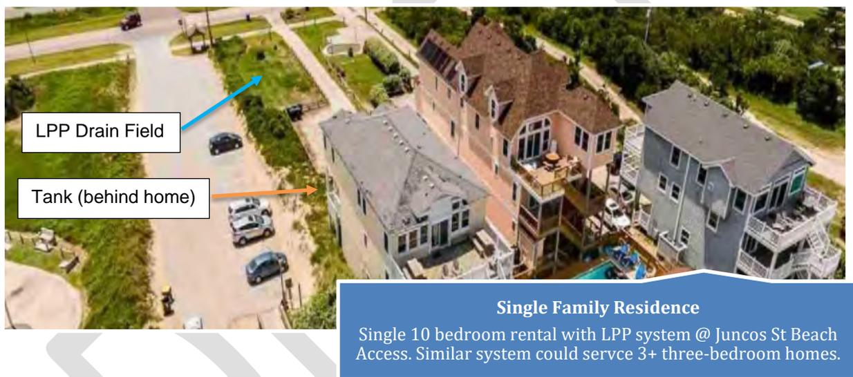
Figure C- 1. Examples of large and/or advanced onsite wastewater systems at large residential sites that provide analogous treatment scale or volume to smaller-scale or clustered residential decentralized cluster system opportunities.
