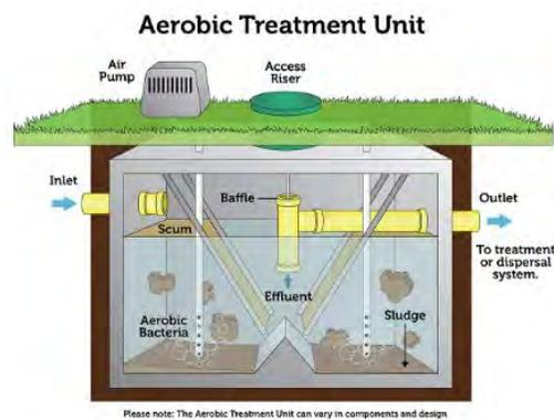
Figure 6-3. Advanced (Aerobic) Treatment Unit, ref. US EPA
