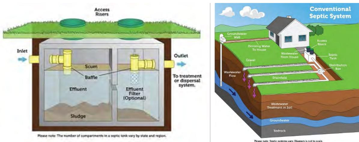
Figure 6-2. Septic tank elevation view (left) and a conventional septic system (right) source: EPA
